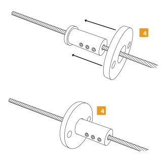
Tighten down set screws on 1.5" round cylinder so the cable is secured.
