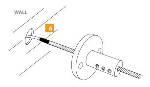
Pull all parts together and mount into the wall with the screws.
